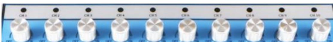
Rotate the corresponding knob to adjust the energy of the pad. After clicking start, the indicator lights on the top of the rotating knobs will be on.
