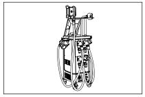
Step 7: Add water. Water drainage: place the funnel at the outlet, and remove it after the tank is completely drained.
