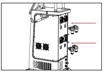
Step 6: Position the applicators onto the holder, and connect them to the main machine.
