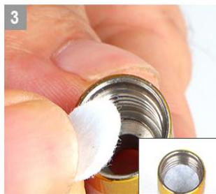
Filter Cotton(A filter cotton must be installed when operating the machine. Otherwise, dirt may enter it, causing damages. Meanwhile, the cleaning effect can be seen.)
