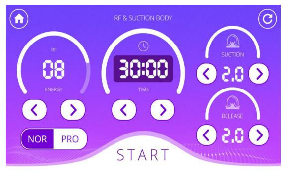
**S**RF energy level and adjusting buttons(3-7 is recommended)
