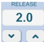
Adjustment for Vacuum Release Time(If it is "0", it is the constant suction mode)
