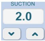
Adjustment for Vacuum Suction Time(suction time is longer than the release time)
