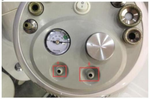
II. Turn the silver knob to adjust the suction of vacuum. Turn to right of the machine, make the vacuum suction at the highest level, turn to left of the machine, vacuum suction is the lowest level.
