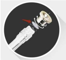
filtering cotton (as what the arrow points at,the filtering cotton must be installed when the treatment is performed to prevent dirt from entering the instrument to cause damage.Additionally, the cleaning effect can be seen with the help of the cotton)
