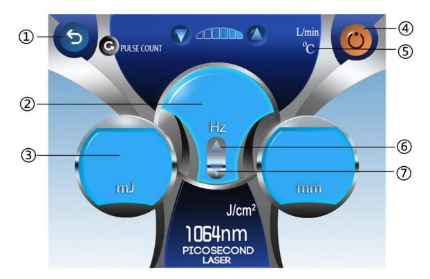
①Return ②Frequency ③Energy ④Start/Pause ⑤Water temperature display ⑥Energy addition adjustment ⑦Energy reduction adjustment
