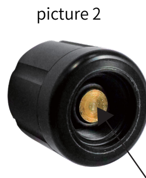
The dent is greater than 2mm and needs to be replaced
