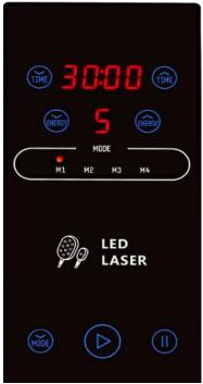
Time Setting & Display of Laser Pad(Time Range: 00: 00 to 60: 00)
