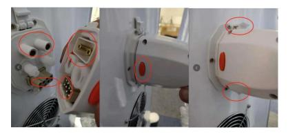
2. Add distilled water: Add distilled water from the injection port until there is water flowing out from the overflow port.
