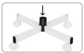
B. Insert the bottom large rod above the black card slot, use a gasket and long screws at the bottom, and tighten it with small wrench.
