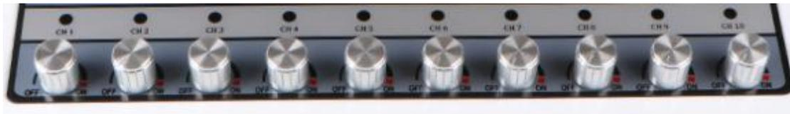
Turn the energy knob of a certain pair of EMS patches and press start button, the light above corresponding knob will be on.
