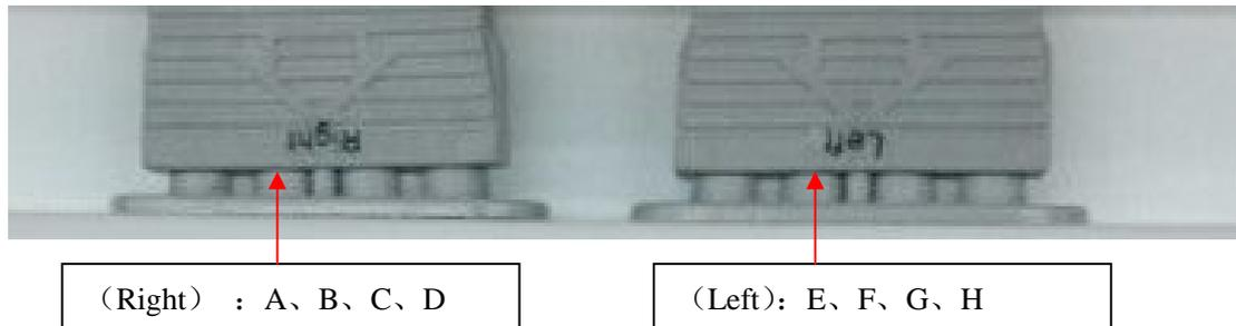
Noted:When connecting to the interface of the instrument, please connect by the indicated direction of sticker (or direction of arrow). Otherwise, the machine can't inflate properly as the indication of the panel. Meanwhile, the inflatable bag (E,F,G,H) of upper body should be connect to the plug(Right), the other A,B,C,D should be connect to the plug(Left).
