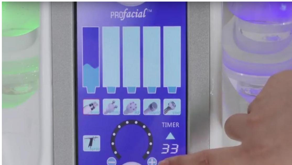
Please rotate the white switch to adjust the vacuum intensity.
