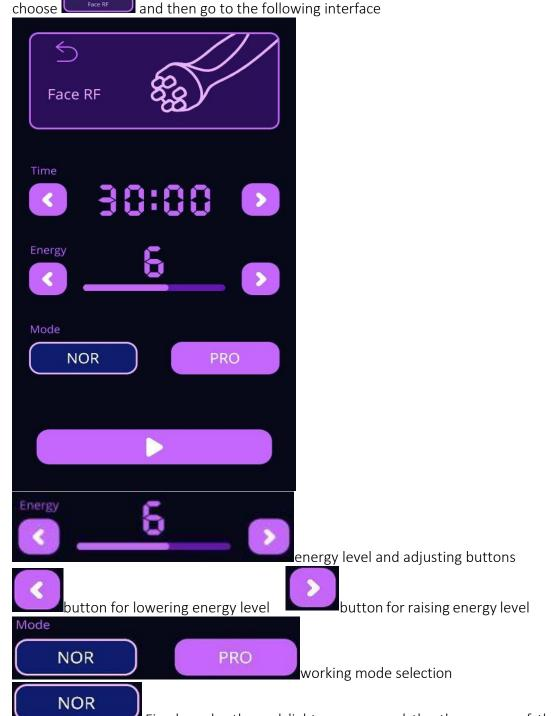
Fixed mode, the red light goes on and the the energy of the handpiece directly reaches preset level after the start button is pressed.
